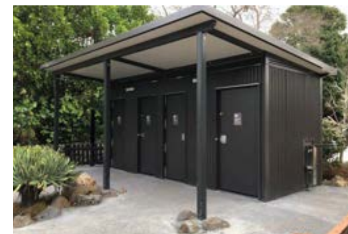
Automatic, DDA compliant toilet unit with unisex, ambulant and disabled cubicles. Consider Colorbond cladding or similar that blends into the environment
